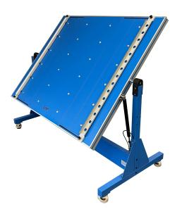
Transfer table with side guides for straight feeding of boards.
